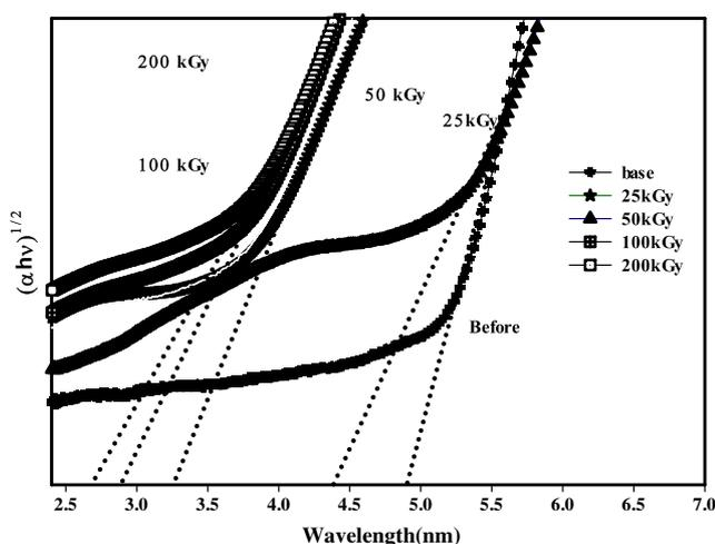
**Fig. 3** Indirect optical band gap determination before and after different doses of gamma irradiation 25, 50, 100 and 200 kGy
