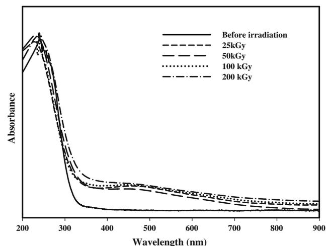
**Fig. 2** Optical absorption spectra of bioactive glass before and after different doses of gamma irradiation
